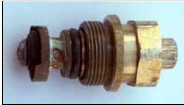
Figure 2.6: Selective Leaching of Brass (www.corrosion-doctors.org)
